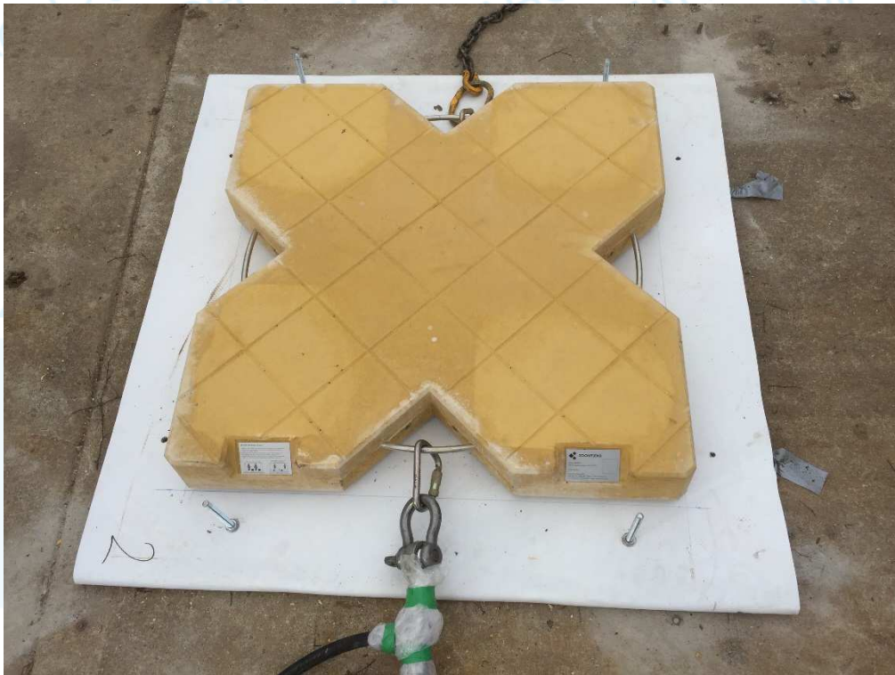
Figure 4 – Anchor device described as “BIBO” (installed on 2 BE using adhesive)
