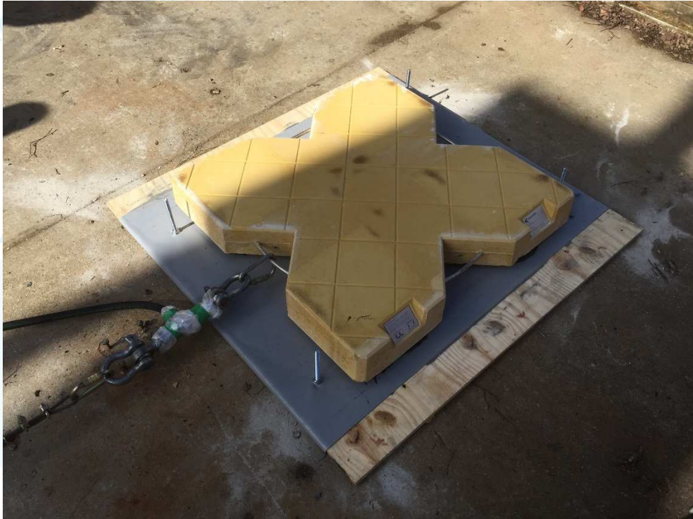
Figure 2 – Anchor device described as “BIBO” (installed on PVC using adhesive)
