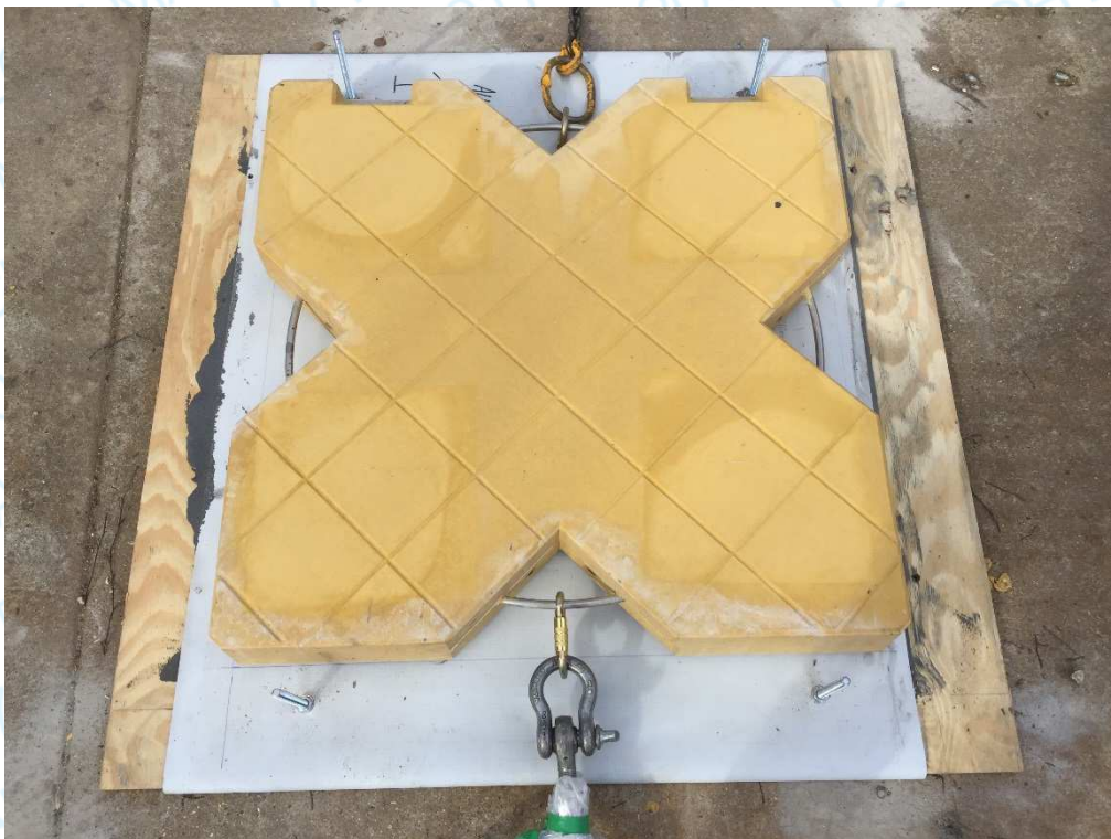
Figure 3 – Anchor device described as “BIBO” (installed on 1 AU using adhesive)
