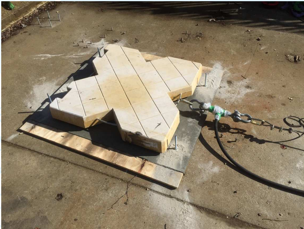
Figure 1 – Anchor device described as “BIBO” (installed on bitumen by heating pads of sample and pressing into roof surface)
